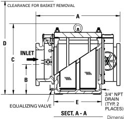
Dimensions and weights are for reference only. Contact Eaton for certified drawings
