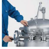
1. Filter element change necessaryopen the safety interlock to ensure simultaneous pressure relief.
